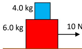
4. There is friction between the 2 blocks. The static coefficient is 0.4. The blocks move as one body. Draw horizontal forces only.
