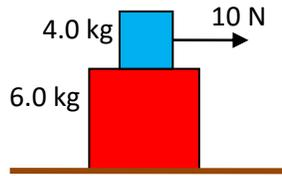
5. The blocks will collide. Label the forces during the collision. Draw horizontal forces only.
